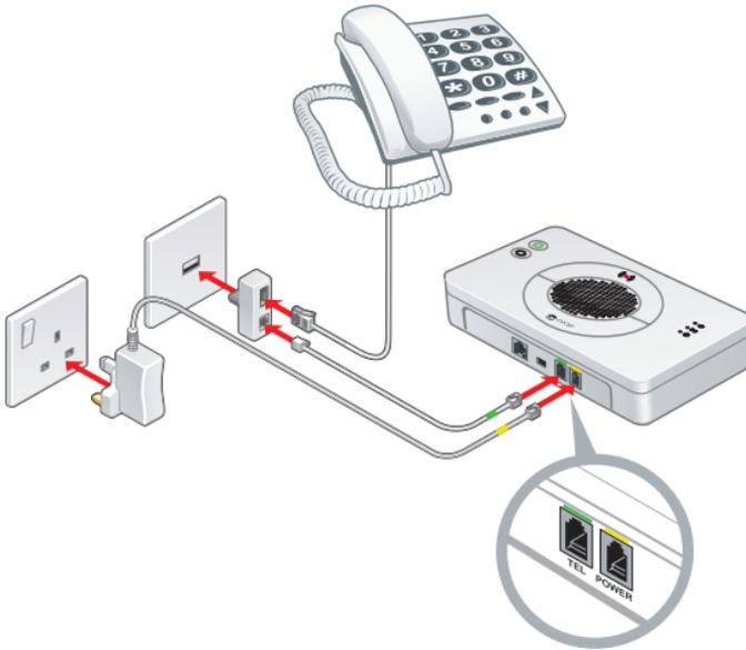
Power is supplied via the power supply from a wall socket.
